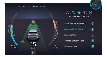
Rush hour pilot adjusts the position of the T10X in the lane and the following distance, providing a comfortable driving experience in heavy traffic with steering support. The driver's attention level is measured with the help of the driver attention assistant with camera, and the system can give a warning or become inactive if necessary. This feature can be used at speeds up to 15 km/h.
